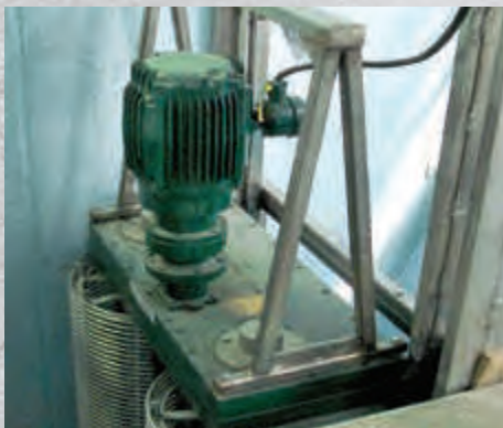
Channel Monster ® with immersible motor and lifting bail.
