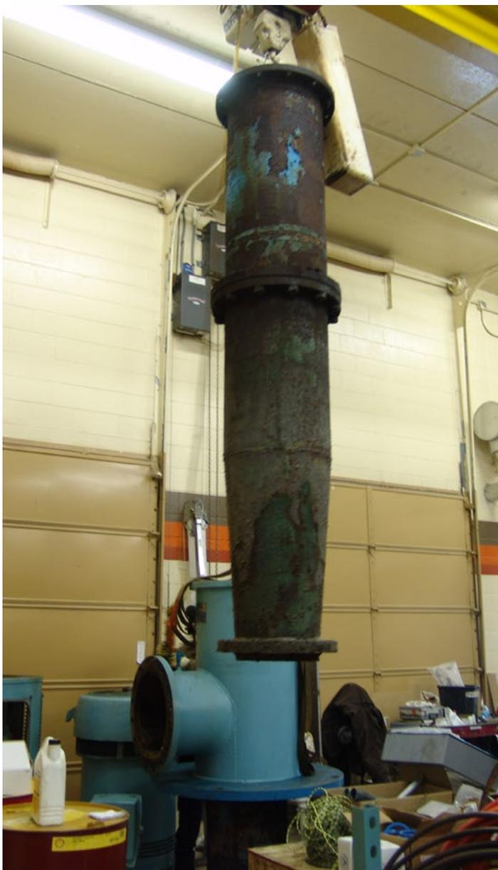
*Large headroom is required for installation and maintenance of vertical turbine pumps. The pump pictured is being removed to be rebuilt after 30 years of service in a clean water application.*
