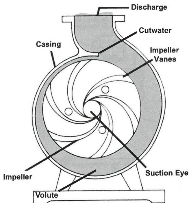
*Illustration from Goulds GPM10, pg 889*
