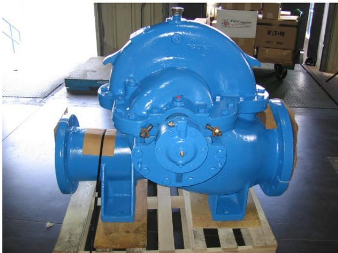
*Rebuilt split case pump from a paper mill.*
