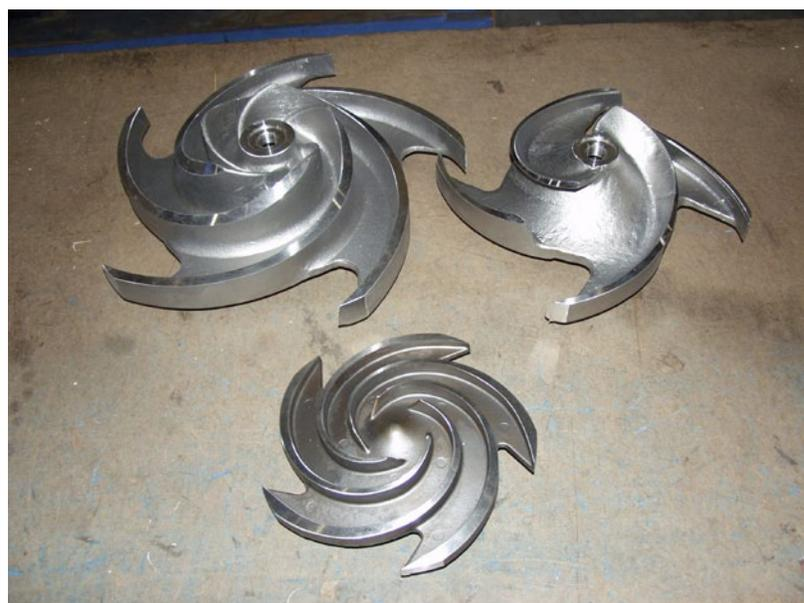
*Examples of open vane impellers.*
