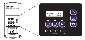
The VSC controller provides integrated control for the 6VSG generator set and programmable interface module (PIM) or communications kit.
