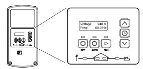
The RDC2 controller provides integrated control for the generator set, Kohler® Model RXT transfer switch, programmable interface module (PIM), and load management device.
